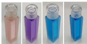
Fig. 4 Cobalt Chloride Solutions (50 °C) Solvents from left to right: pure water, methanol, ethanol, and acetone
