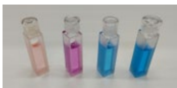
Fig. 1 Solutions of Cobalt Chloride Solvents from left to right: pure water, methanol, ethanol, and acetone
