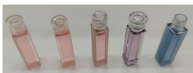
Fig. 7 Solutions of Cobalt Chloride (Room Temperature) Pure water to acetone solvent ratios from left to right: 1:1, 1:2, 1:3, 1:4, and 1:5
